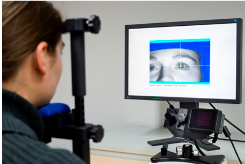
Figure 33. Adjusting head position with eye tracker
